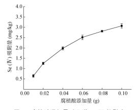
图 5 腐植酸添加量对吸附 Se(IV)的影响 Effort of hymic soid additive amount on Se(IV) add
