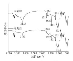
图 2 腐植酸吸附 Se(IV)前后的红外光谱图 Fig. 2 FTIR spectra of humic acid before and after adsorption of Se(IV)
